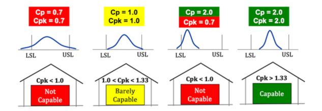
Now ,Let us first conduct process capability analysis on input using Python, we have two input variables 1.Shaft diameter = d ,2.Hole diameter=H and one output variable i.e. Y= fitment class.
